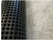
A UV stabilised geotextile layer filter, thermally bonded on one side of a cuspated HDPE core, suitable for both active and passive venting systems. Its main application is to remove gases such as Radon, Methane, Carbon Monoxide, Hydrogen Sulphide etc. from below base slabs of offices, industrial and commercial buildings.
