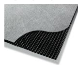
A geocomposite drainange layer comprising high performance second generation single cuspated HDPE (High Density Polyethylene) core with a geotextile filter thermally bonded on one side. The textile filter has a flap extending beyond the core on one edge. The major application is its use instead of stone drainage layers in landfill containment systems.
