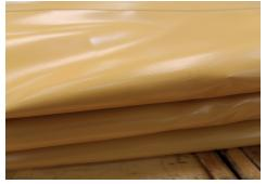
This cloth reinforced PVC geomembrane possesses a greater puncture resistance than plain unreinforced polymers due to the multi-ply nature of the material with 2 layers of polymer, one on either side of the high tenacity base cloth. The high tensile strength of the polyester material gives the geomembrane a very tough tear strength and with the good adhesion properties of the polymer to the cloth, offers excellent resistance to mechanical damage.
