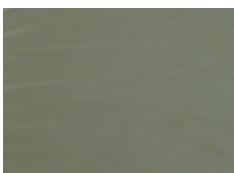
This cloth reinforced PVC geomembrane possesses a greater puncture resistance than plain unreinforced polymers due to the multi-ply nature of the material with 2 layers of polymer, one on either side of the high tenacity base cloth. The high tensile strength of the polyester material gives the geomembrane a very tough tear strength and with the good adhesion properties of the polymer to the cloth, offers excellent resistance to mechanical damage.
